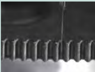
Measuring form of micro gear teeth
