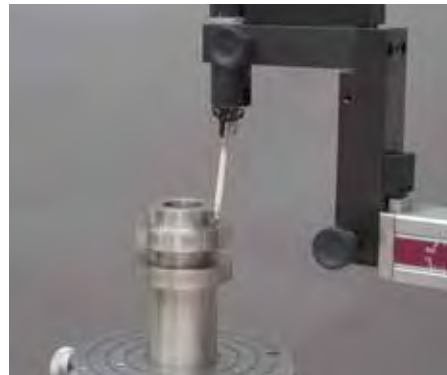
Spiral-mode cylinder measurement
