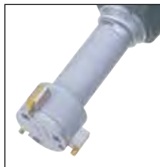
TiN-coated contact points (" -10" suffix models only)
