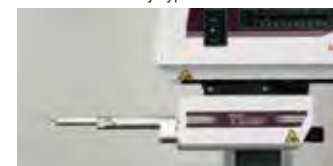
178-076 (S-3000MR) Manual Rotary Type Detector Holder
