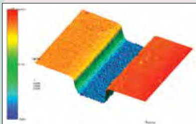
3-dimensional topographical result, data of micro-circuit
