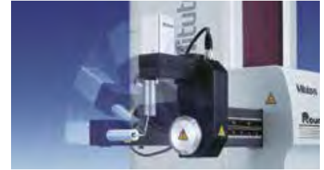
Holder-arm orientation switching (vertical position - horizontal position)
