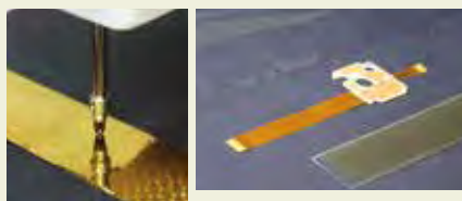
Thickness measurement of non-metallic sheet
