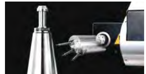
Detector rotation mechanism (0 to 290°, in increments of 1°)
