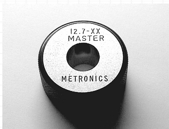
Metronics 12.7mm Sharp Edge Ring Gauge (with magnified view of the top plane)
