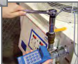
...into a highly accurate digital torque tool.
