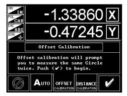
Figure 14 Offset Calibration between the Fiber-Optic Cable and the Crosshair
