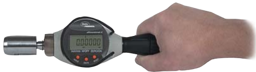
The μDimensionair is the ultimate of portability and versatility – in your hand or at the workbench or machine tool. Shown with optional 2239307 Bench Kit
