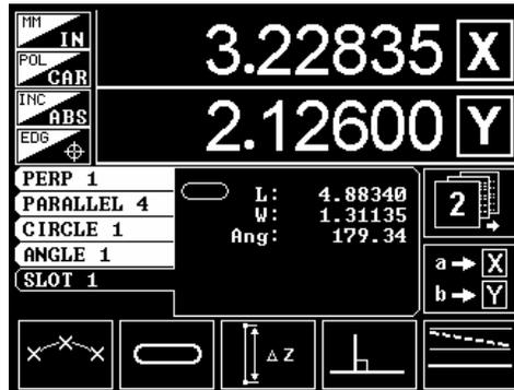
**Figure 37 DRO screen showing a Slot measurement**
