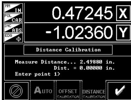
**Figure 18 Distance Cal Step Two**
