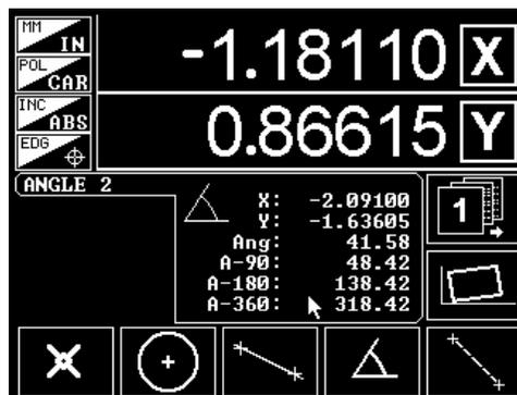
Figure 31 DRO screen showing an Angle
