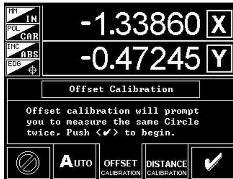
**Figure 14 Offset Calibration between the Fiber-Optic Cable and the Crosshair**
